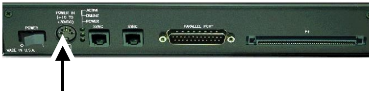
DIN5 POWER IN Connector (+10 to +30 VDC)
